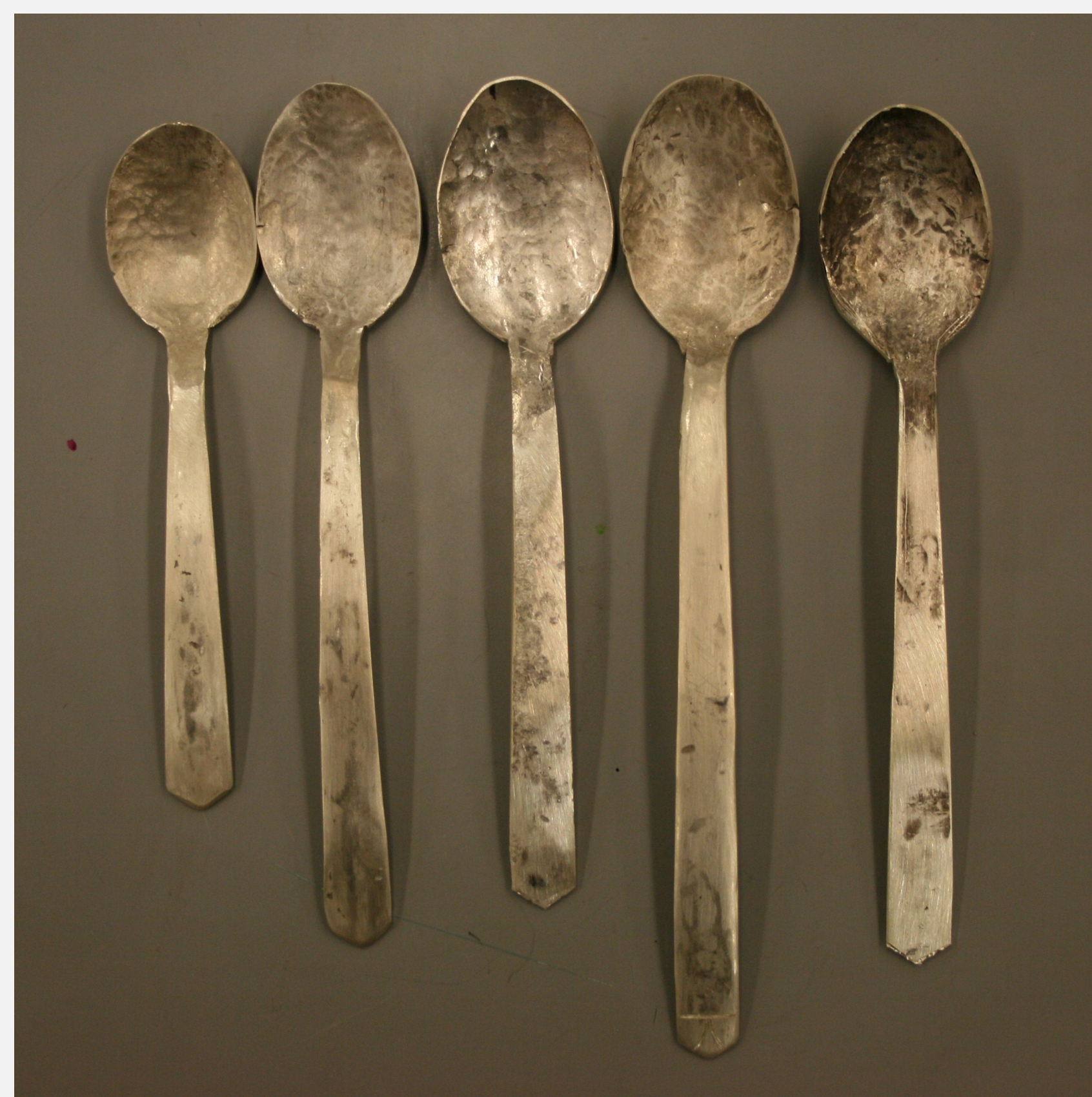
Figure 1: spoons, respective copper content (processes), left to right: 4.5% (rolled), 4.5% (forged); 7.5% (rolled); 7.5% (forged); 9.5% (rolled).
